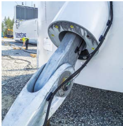
TRUpin - continuous measurement and monitoring of rope forces.
