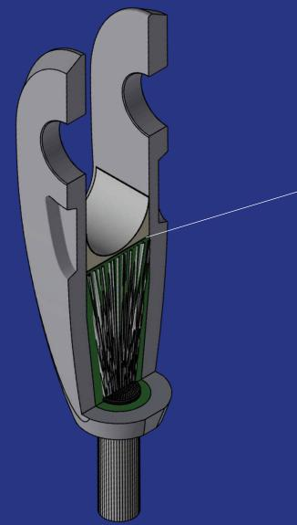
The interlayer positioned between TRUlock and the spelter socket allows for cone setting without affecting the cover layer.
