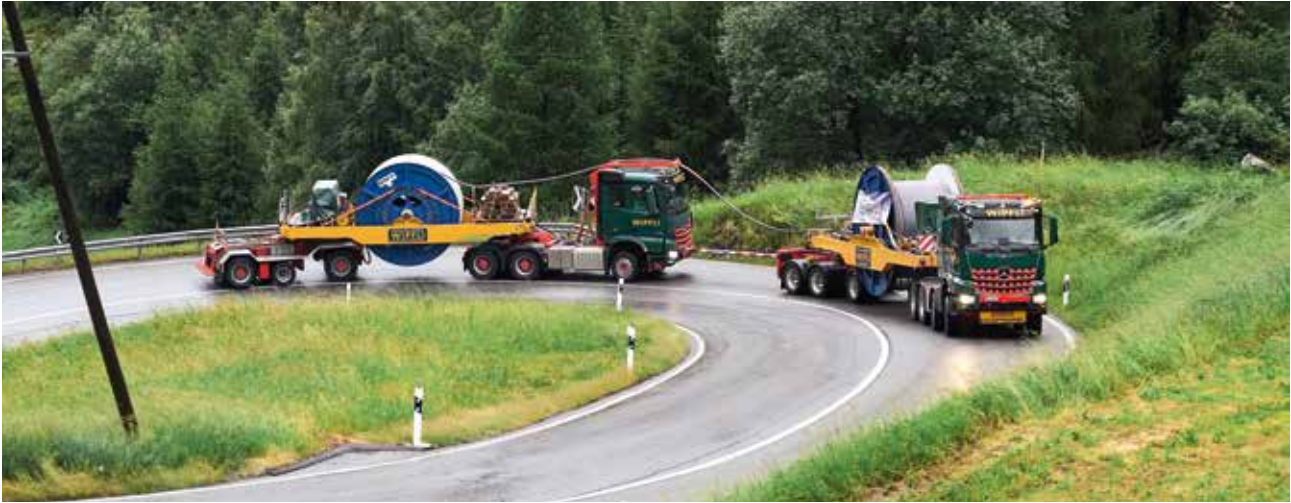
Mountainous regions often involve the need to overcome tight curves and limited load-bearing bridges. The ropes are therefore distributed among several carriers with these types of heavy loads.
